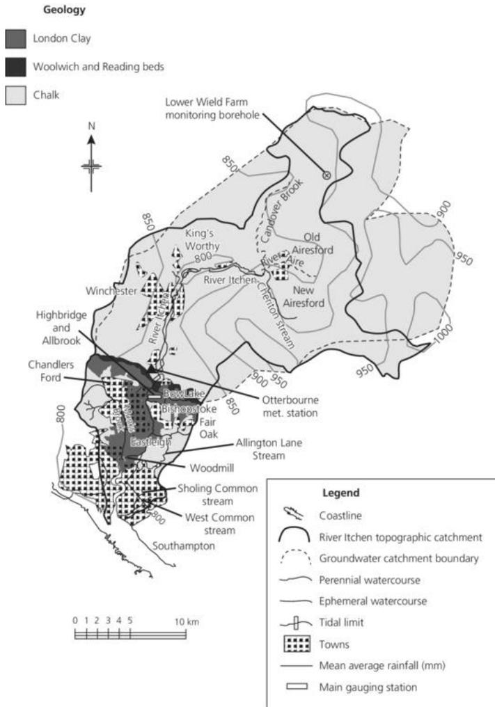
**Figure 2.6** Surface and groundwater catchments on the Itchen. (Redrawn from NRA, 1992e, p. 12).
