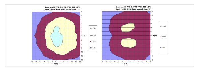
Figure 7: LumenArc III: Par distribution top view, 24" and 30".
