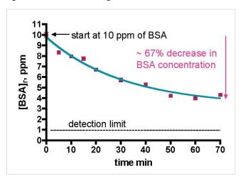
Figure 8. BSA depletion in freshly prepared saltwater using the Euroreet CS80 skimmer. The green line is the best fit using Eq. (21).
