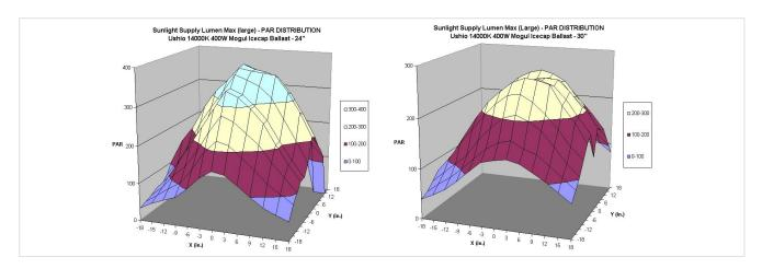
Figure 11: LumenMax (large): Par distribution side view, 24" and 30".
