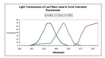
Figure 1. Approximate transmission qualities of three colored filters used by D'Angelo et al. (2008).
