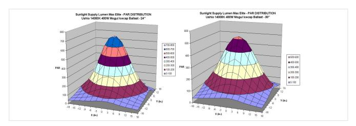
Figure 2: LumenMax Elite: Par distribution side view, 24" and 30".
