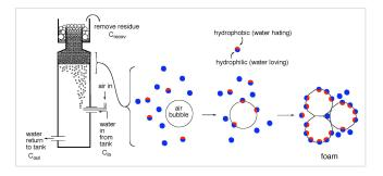
Figure 1. Schematic of the skimming process.
