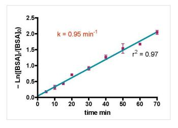
Figure 9. Mathematical treatment of the Euroreef CS80 data in Fig. 8 using Eq. (20) with Q = 2.9 gpm,  $V_S$  = 0.62 gallons, and  $V_r$  = 35 gallons.
