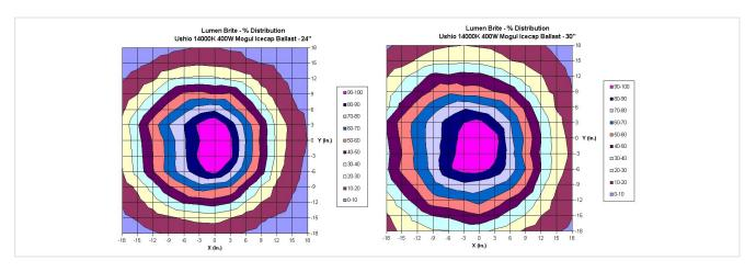
Figure 6: LumenBrite III: Par distribution percent, 24" and 30".
