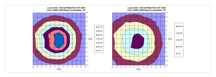
Figure 4: LumenBrite III: Par distribution top view, 24" and 30".
