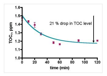
Figure 11. A second attempt to measure TOC depletion in authentic aquarium water using the Euroreef CS80 skimmer. The water sample was removed from the aquarium 1 hour after feeding. The green line is the best fit using Eq. (21).
