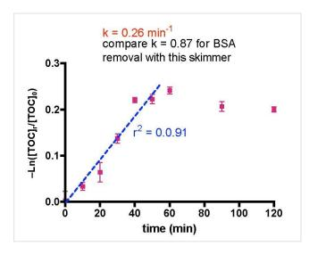
Figure 12. Mathematical treatment of the data in Fig. 12 using Eq. (20) with Q = 2.9 gpm,  $V_{\rm S}$  = 0.62 gallons, and  $V_{\rm r}$  = 30 gallons.
