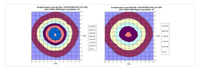
Figure 1: LumenMax Elite: Par distribution top view, 24" and 30".
