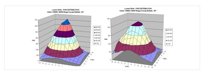
Figure 5: LumenBrite III: Par distribution side view, 24" and 30".
