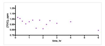
Figure 10. A first attempt to measure TOC depletion in authentic aquarium water using the Euroreef CS80 skimmer. The water sample was removed from the aquarium 24 hours after feeding.
