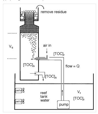
Figure 5. The skimmer/reservoir system used for derivation of the math that leads to k, the rate constant for TOC removal.
