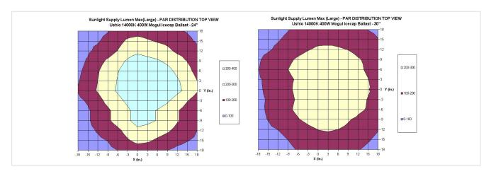
Figure 10: LumenMax (large): Par distribution top view, 24" and 30".
