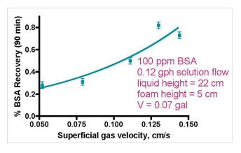
Figure 2. Skimmer performance as a function of gas flow rate (from Brown, 1990).
